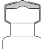
**Upward bulge of the crimp cap**
